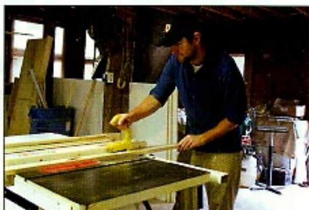
Doing it all — The jet table saw that Luke Bowers is using does all the ripping and cutting in the shop. Mike Bowers believes that it's best to keep tools simple.
